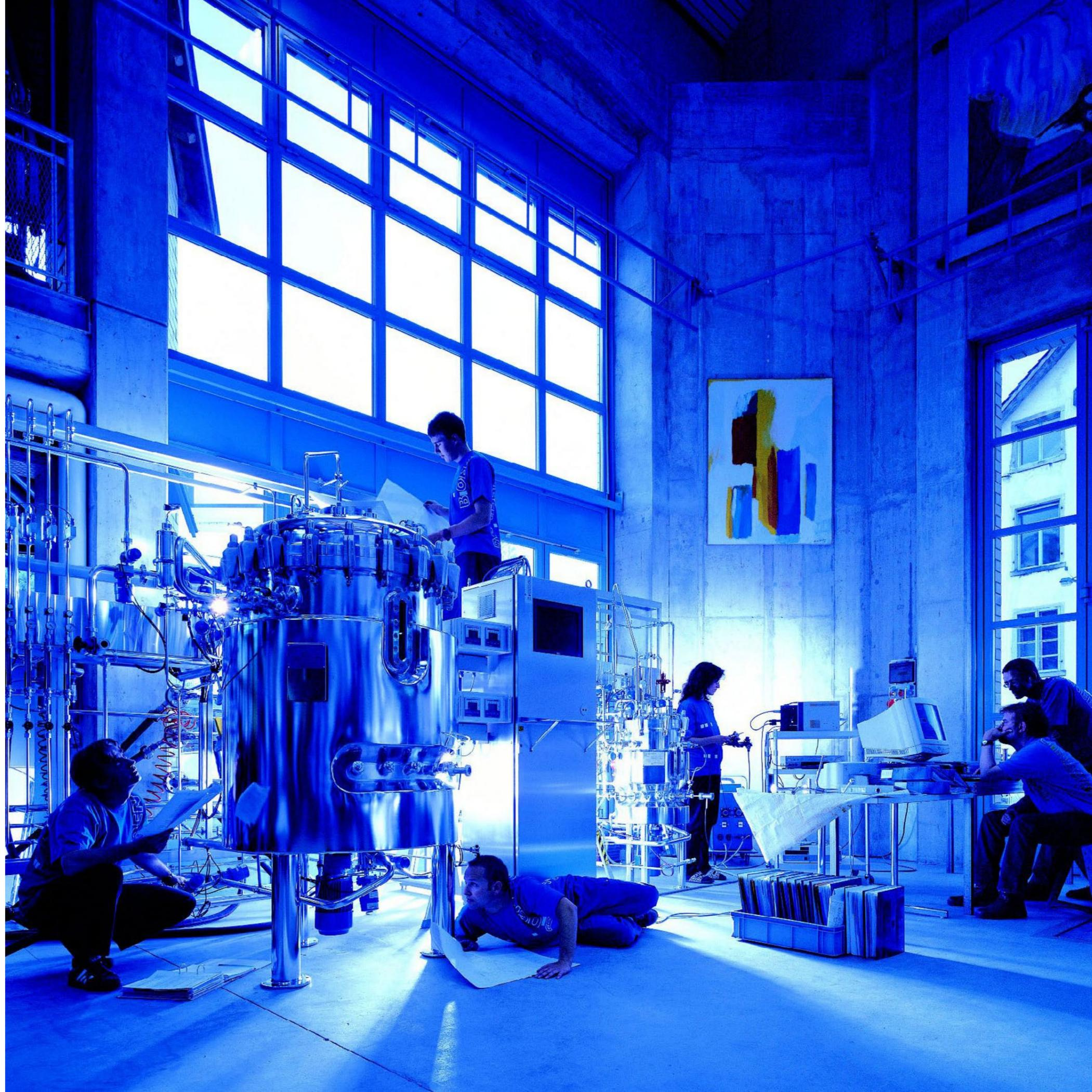
The Factory Acceptance Tests (FATs) required by the pharmaceutical industry today are conducted in our manufacturing facilities with an infrastructure consisting of space, water, steam and power as well as service rooms and personnel. Against payment, we will assist customers in obtaining the certifications required by the regulatory authorities. This example involves a Factory Acceptance Test (FAT) conducted on behalf of a customer for a cell culture fermentation plant.
